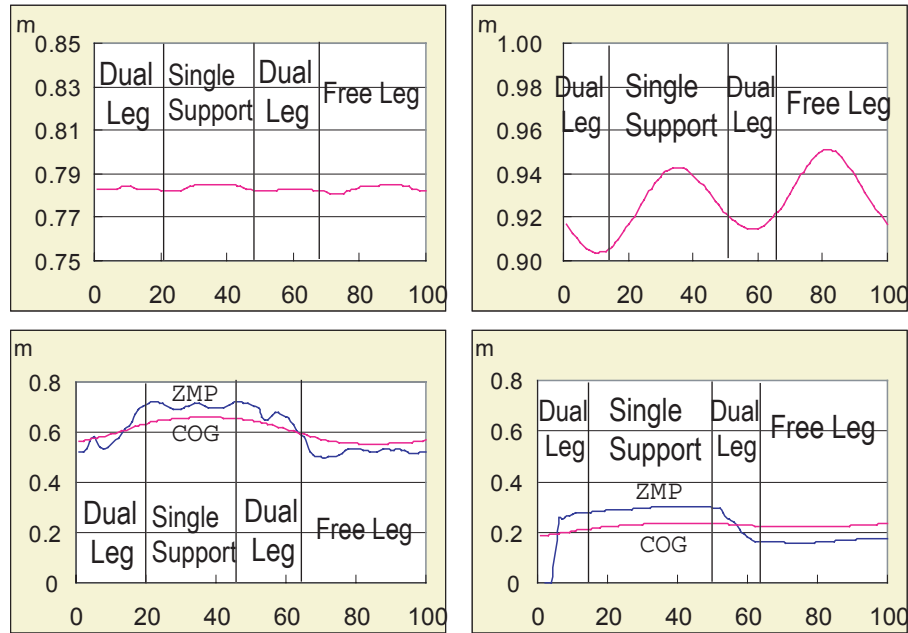
Fig. 4. Sagittal Movement of Center of Gravity (upper) and Lateral Movement of CoG/ZMP (lower): H7 (left), Human (right)
