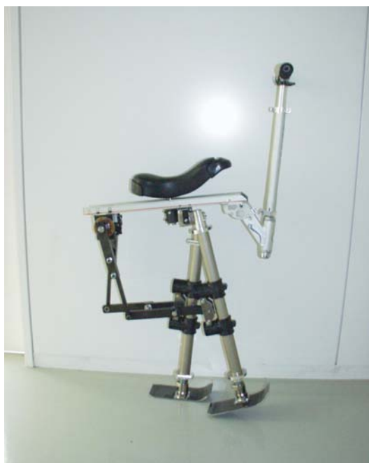
Fig.4 The prototype of the powered passive bipedal walker with the saddle
