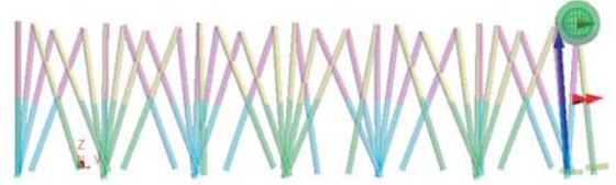
Fig. 3: Biped walking simulation by “multi-trajectory shifting control” with memory based push off control
