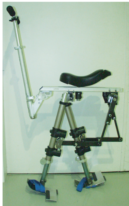
Fig.1 The prototype of the human powered passive bipedal walker with the saddle
